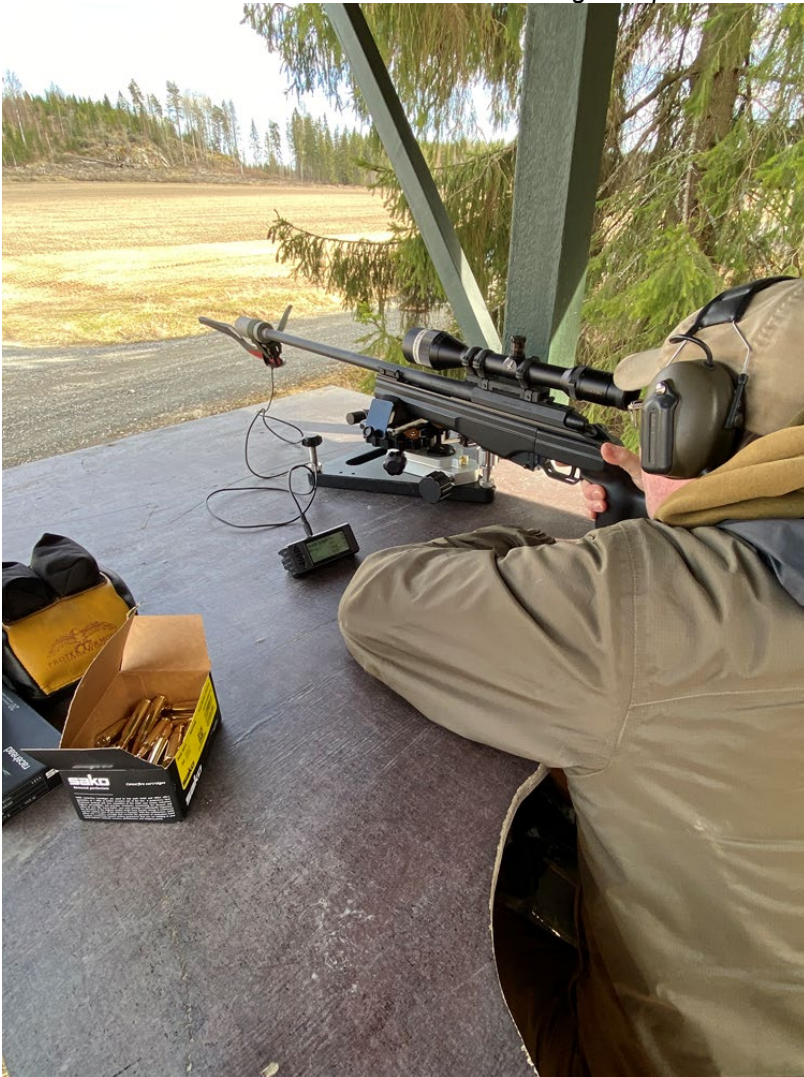
Pic 1. Bullet velocities were measured with a magnetospeed V3 ballistic chronograph.
